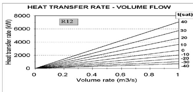
Figure 5. Heat transfer rate versus volume rate.
