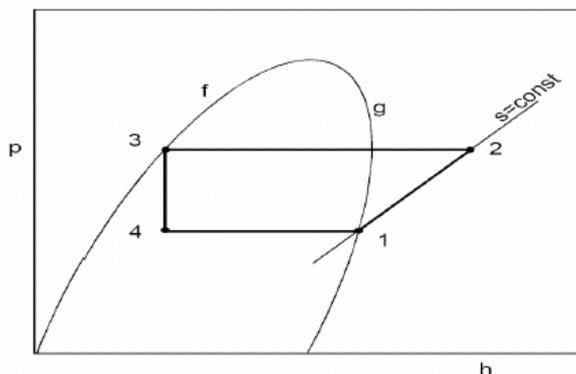
Figure 14. Refrigeration cycle.
