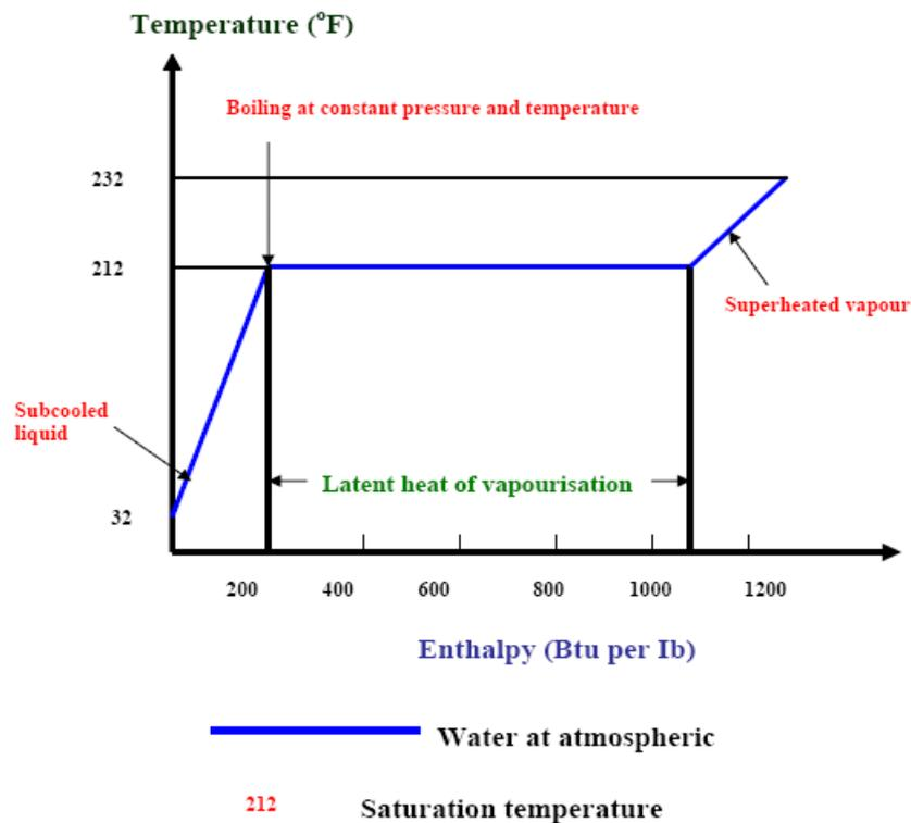
Figur 13. Water undergoing a charge of state.
