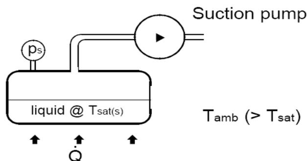
Figure 4. Refrigeration Cycle.
