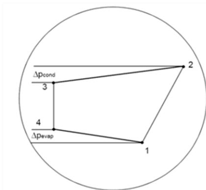
Figure 18. Pressure drops in evaporator and condenser.
