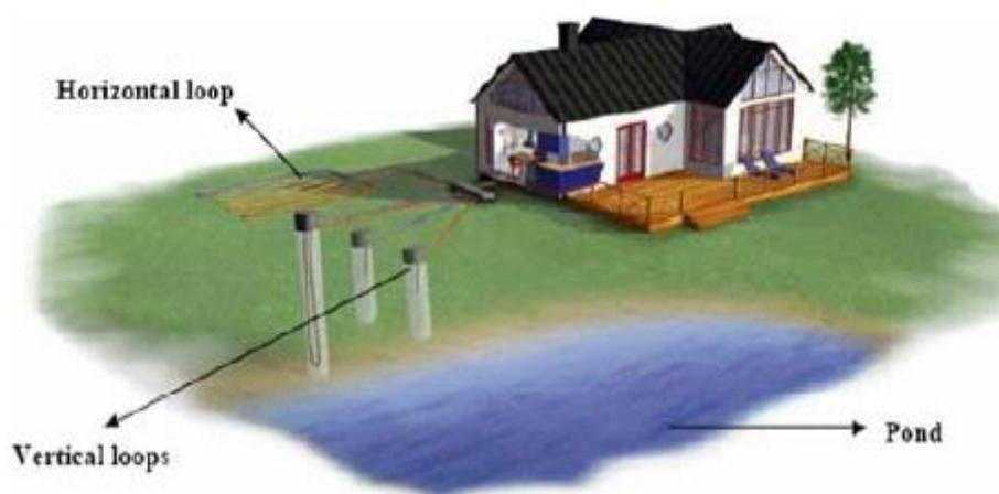
Figure 1. Using the soil, bedrock or groundwater as the heat source [17].
