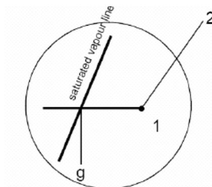
Figure 15. Evaporator superheat.
