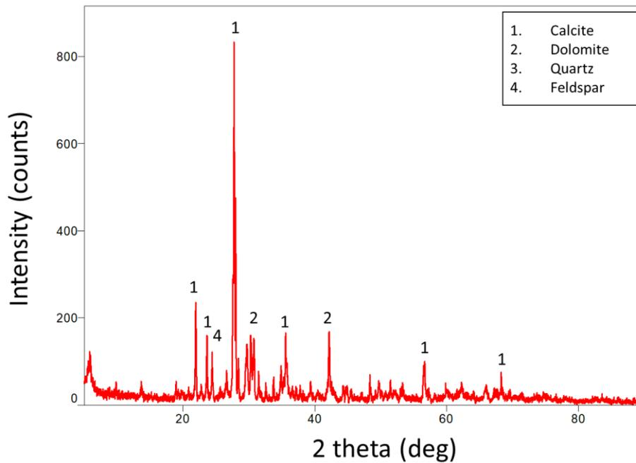
Figure 2: XRD spectra of black aggregate
