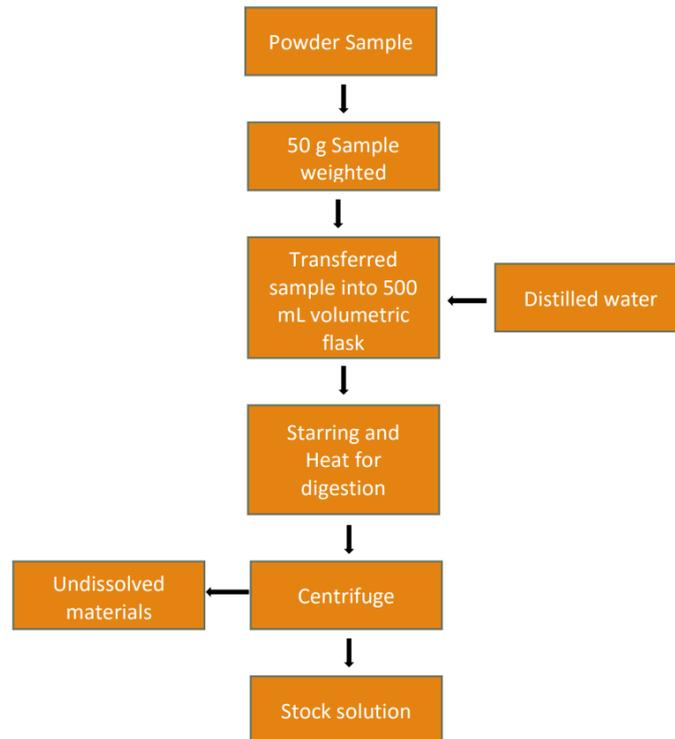
**Figure 1: Block diagram presentation for aqueous stock solution preparation technique.**
