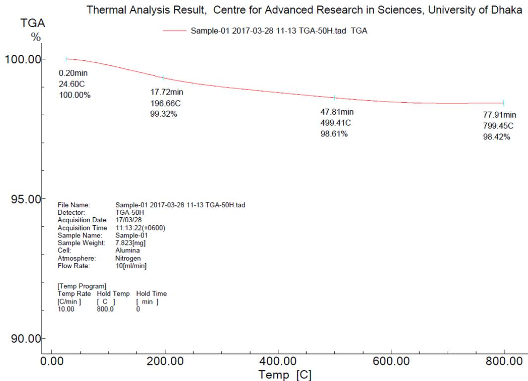
Figure 4: TGA image of black aggregate
