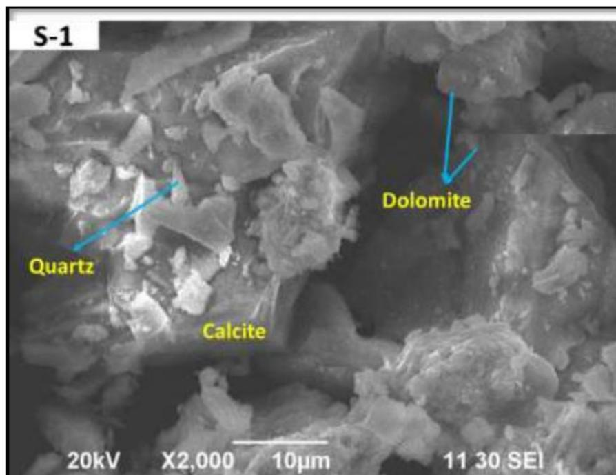
Figure 3: SEM image of the black aggregate
