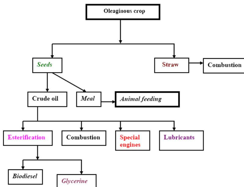
**Figure 9. Flow chart of biodiesel production (Omer, 2006).**
