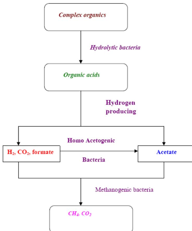
**Figure 3. Biogas production process (Omer, 2003).**
