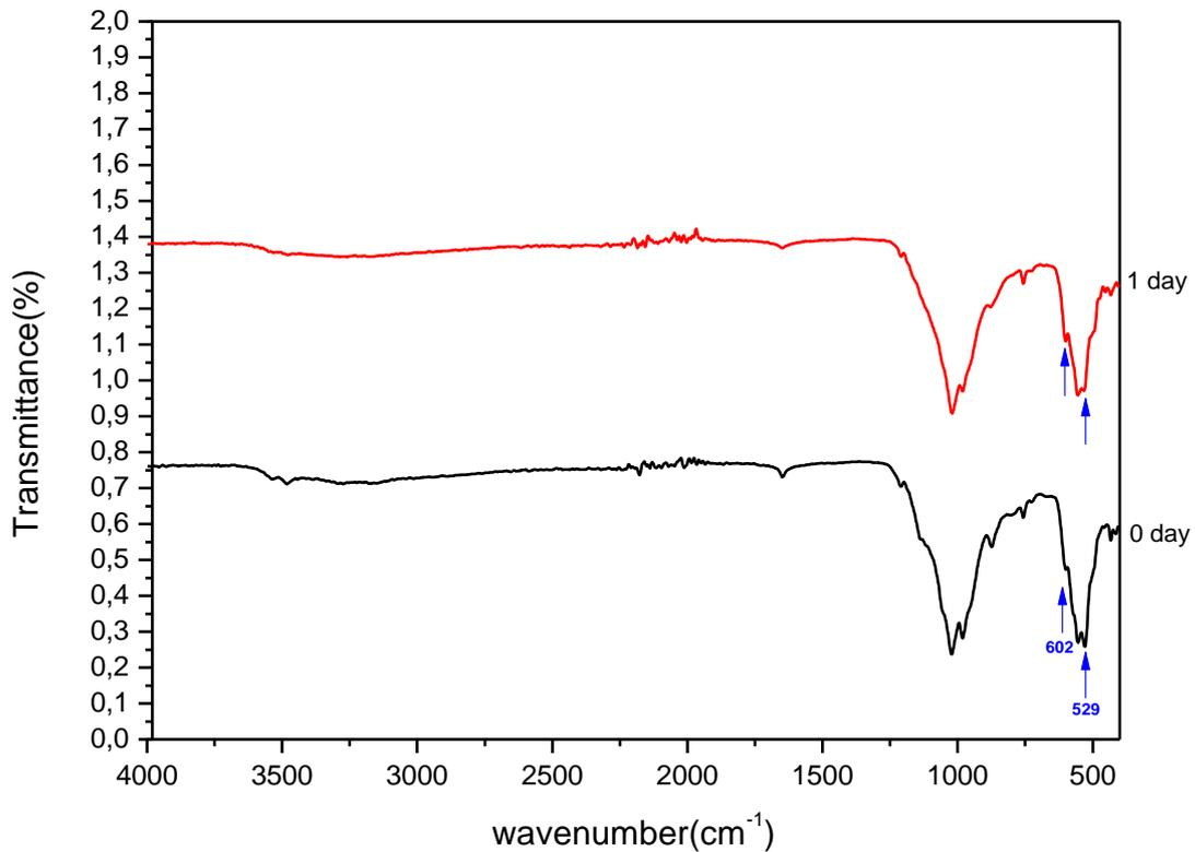
**Figure 2.** The FTIR spectrum of cement after soaking in water for: 0 and 1 day
