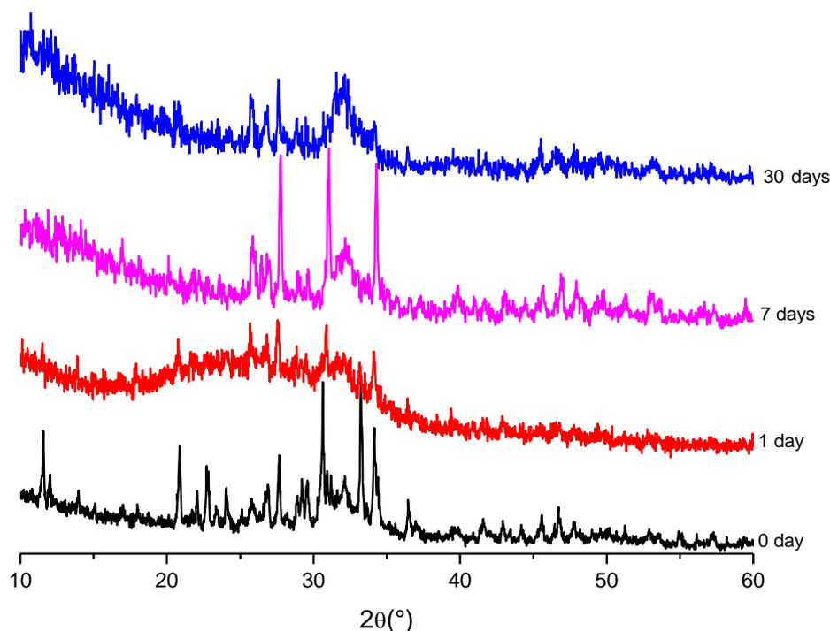
**Figure 1. The XRD patterns of cement after soaking in water for: 0, 1, 7 and 30 days**
