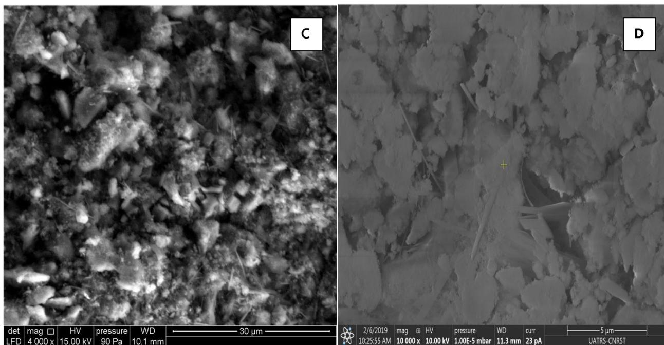
**Figure 3. The SEM micrographs of fractured surfaces of cements soaking in water for: (A) 0 day, (B) 1 day, (C) 7 days and (D) 30 days**
