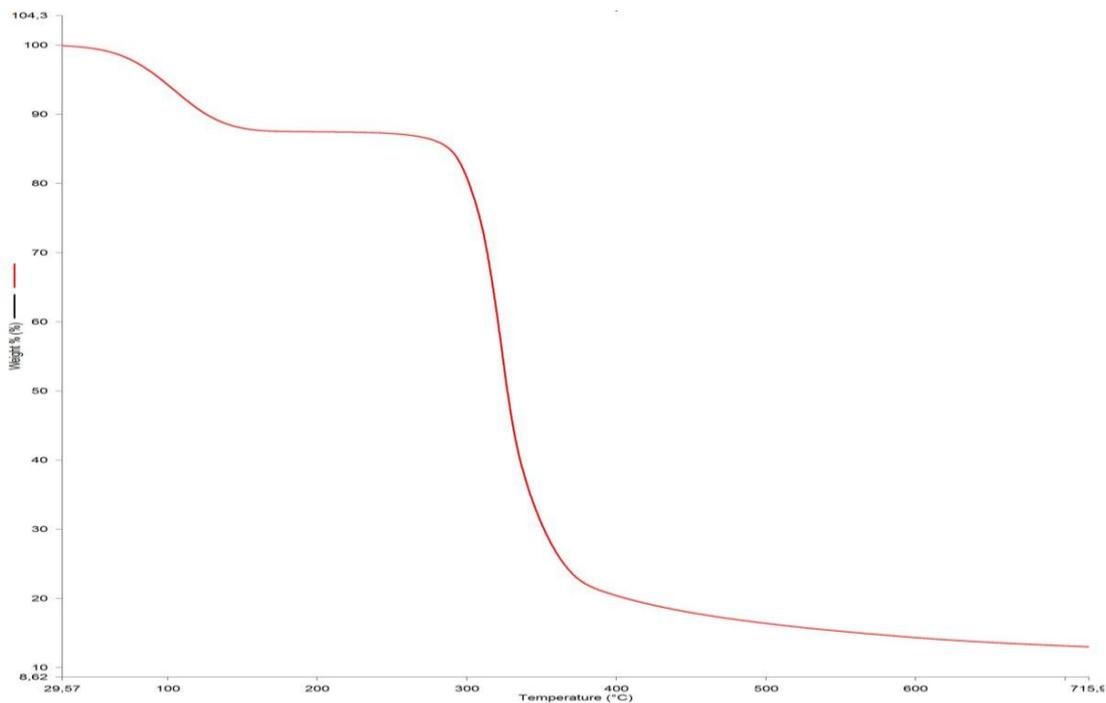
**Figure 4(a):** Thermo-gravimetric Analysis (TGA) Spectrum of Modified Poly (ester amide)
