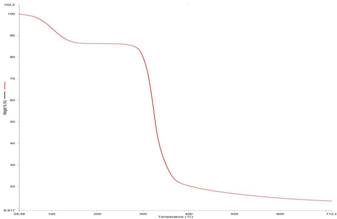
**Figure 3(a):** Thermo-gravimetric Analysis (TGA) Spectrum of Unmodified Poly (ester amide)
