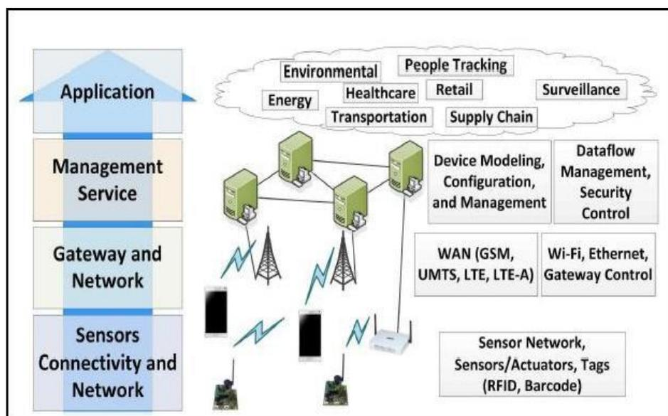
Figure 1: Architecture of IOT
