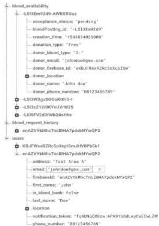
Fig. 10. Firebase database structure
