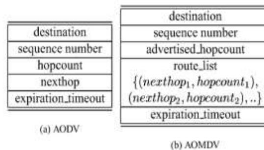
Fig.1 Structures of Routing Table
