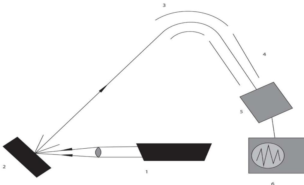
**Figure 3.** Scheme of a time-of-flight mass spectrometer with a laser-plasma ion source: 1 – laser, 2 – irradiated target, 3 – electrostatic analyzer, 4 – drift length, 5 – registration system of ions, 6 – oscilloscope.
