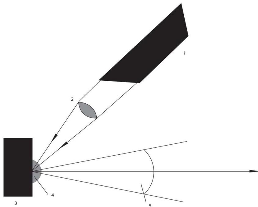
**Figure 1.** Scheme of a laser-plasma ion source: 1 – laser, 2 – focusing lens, 3 – target, 4 – laser plasma, 5 – ion beam having a maximum charge and maximum energy.
