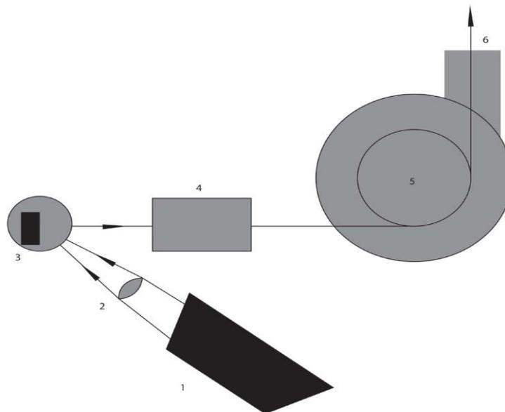
**Figure 2.** Scheme of the acceleration of carbon nuclei at the proton synchrotron using a laser-plasma source of carbon nuclei  $C^{6+}$ : 1 – laser, 2 – lens, 3 – graphite target, 4 – linear accelerator, 5 – synchrotron, 6 – output beam.
