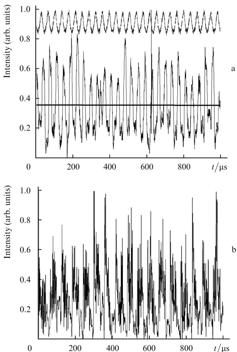
**Figure 4. Rough pulse temporal structures of laser radiation for a modulation Depth-3% and A modulation frequency of-27KHZ (top-modulating Signal, Bottom-output laser signal) (a) and for a modulation depth of 7% and a modulation frequency of -25KHZ(b)**
