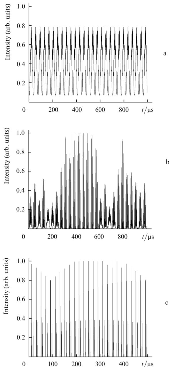
**Figure 3.** Rough pulse temporal structures of output laser radiation for a modulation depth of 5% and a modulation frequency of 27 kHz (a), 5.8% and 27 kHz (b), and 5% and 50 kHz (c);  $M = 1.45$ .
