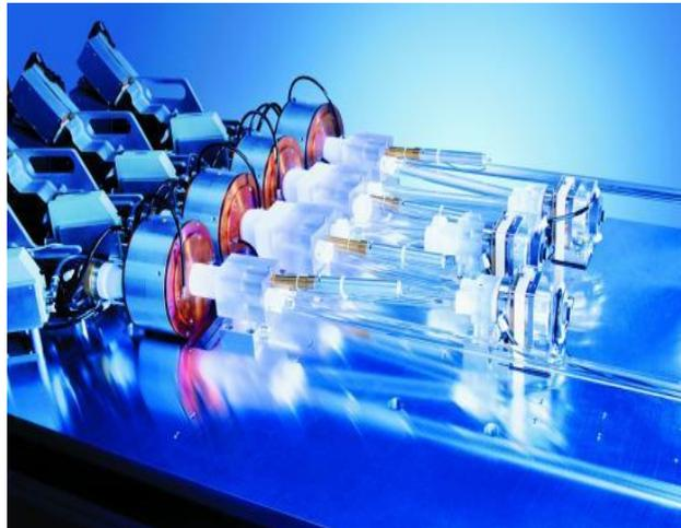
**Figure 6.** " Zig-Zag" disk Laser consisting of a series of disk modules in a single cavity (TRUMPF [5]).
