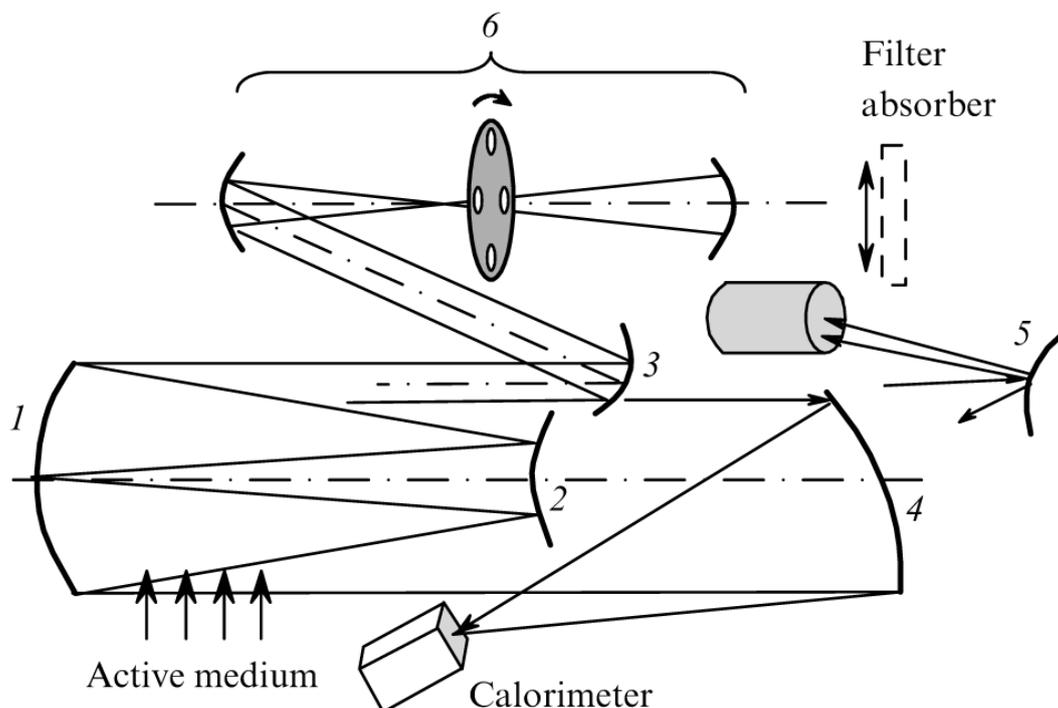
**Figure 1.** Scheme of the experimental setup: (1, 2) mirrors of the unstable resonator; (3) mirror coupler; (4) rotatory mirror; (5) deflecting mirror; (6) system for the formation of an injected beam.
