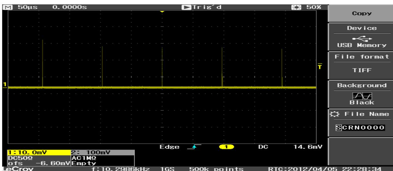
**Figure 5.** High repetition rate P-P mode of operation for high power Nd YAG laser.
