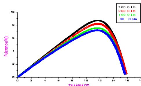
The effect of the shunt resistor is light on the characteristic curve of the panel. We will note that there is a slight variation of  $I_{sc}$ . On physically  $R_{sh}$  interpreter carrier recombination, that is to say the decrease in the phenomenon of recombination depends on the increase of  $R_{sh}$ .
