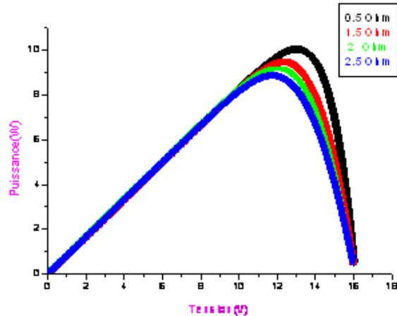
Fig.11: the influence of the series resistance on the characteristic  $P(V)$  for the panel tandem
