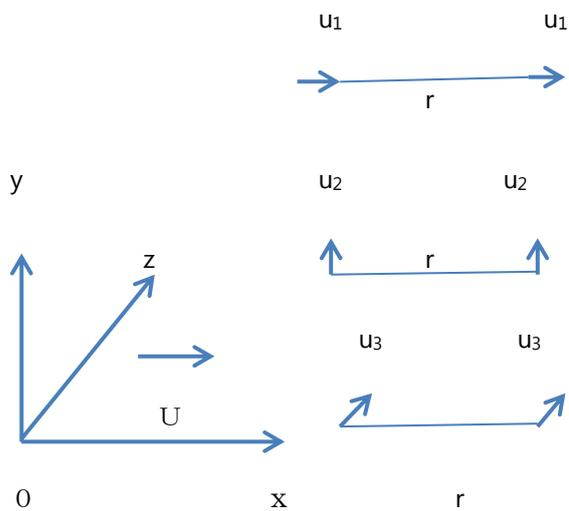
Figure 3 Sketch for explaining longitudinal and transverse double velocity correlations.
