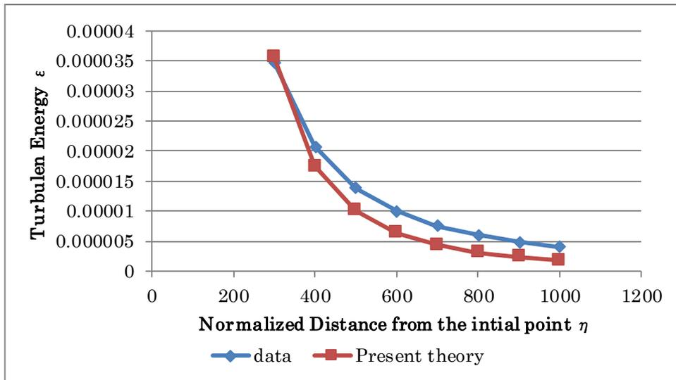
Figure 2: Turbulent energy  $\epsilon = \langle \Delta u \rangle^2 / U^2$  against normalized coordinate  $\eta = x/M - x_0/M$  in the main flow direction.
