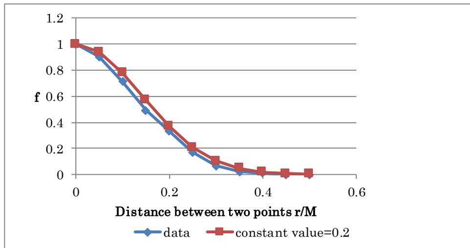
Figure 1: Longitudinal Double velocity correlation function  $f$  against distance between two points  $r/M$ .
