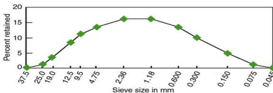
**Figure 2:** Optimum Combined Aggregate Grading for Concrete
