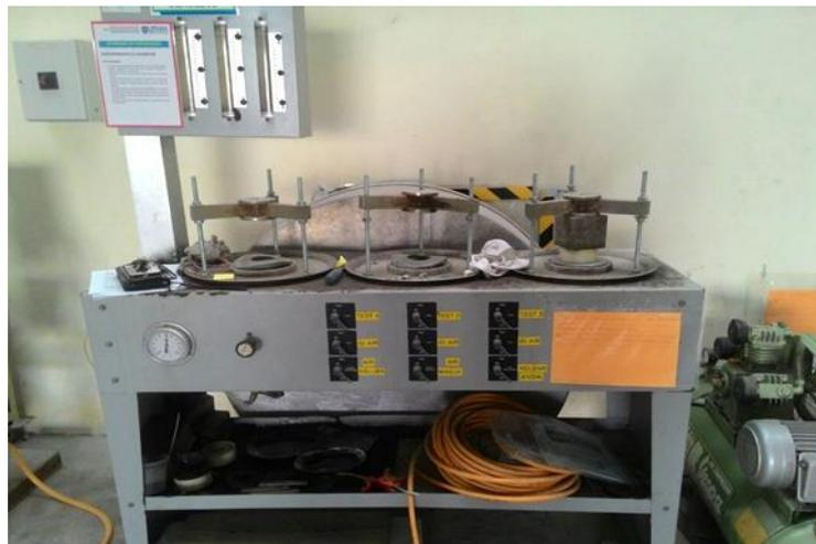
**Figure 3:** Concrete Permeability Test Machine
