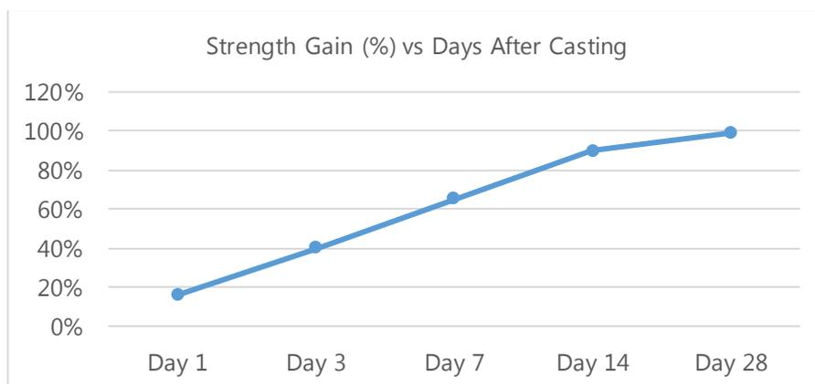
**Figure 7:**Percentage of strength gain vs days after casting
