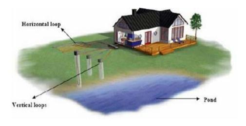
Figure 1. Using the soil, bedrock or groundwater as the heat source [17].
