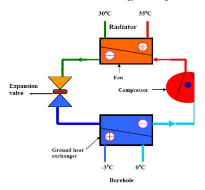
Figure 2. Detail of the GSHP circuit.
