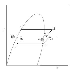
Figure 21. Cycle of multiple compressions using flash chamber.
