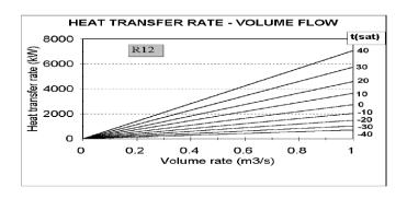
Figure 5. Heat transfer rate versus volume rate.
