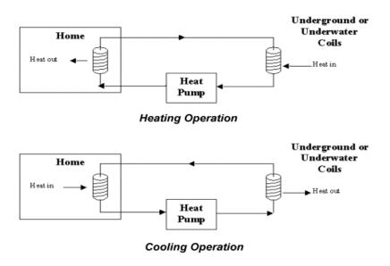
Figure 10. Heating and cooling operations.
