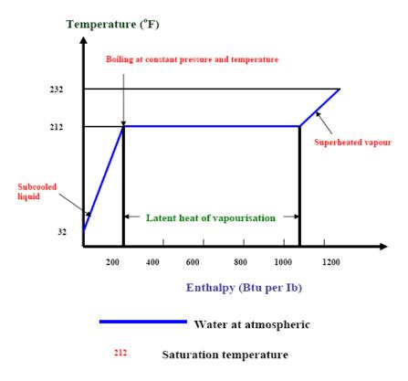
Figur 13. Water undergoing a charge of state.
