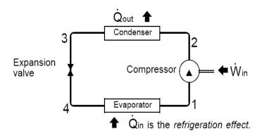
Figure 7. Simplified refrigeration system diagram.
