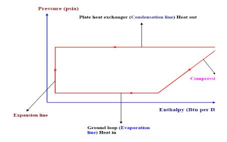
Figure 12. The ideal cycle on Pressure-Enthalpy diagram.
