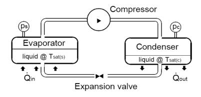
Figure 8. Heat pump refrigeration cycle.
