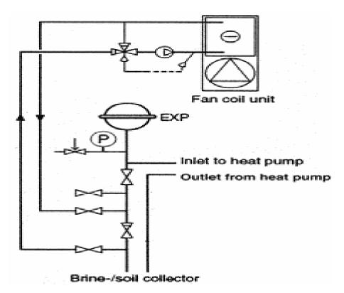
Figure 3. Diagram of cooling system.
