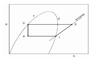
Figure 14. Refrigeration cycle.
