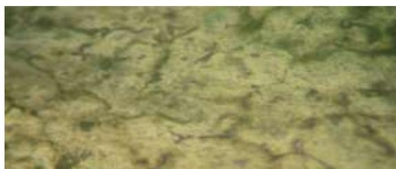
**SAMPLE B** The grain boundaries were reduced with the addition of Cu. (2.5%)
