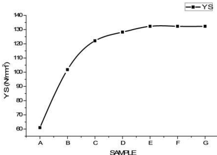
**Fig. 3.2 A graph of Yield strength against copper concentrations of aluminum and aluminum copper designated samples A to G.**
