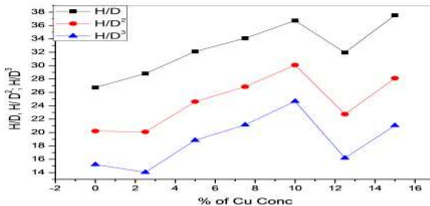
**Fig. 3.5: Combined graph of H/D, H/D<sup>2</sup> and H/D<sup>3</sup> against % concentration of Cu for the designated samples**
