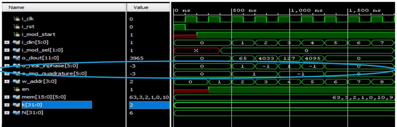
**Fig.5. Output waveform of a QPSK Modulation mapping.**
